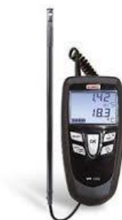
The hot-wire probe used in the measuring of the experimental data [9]
